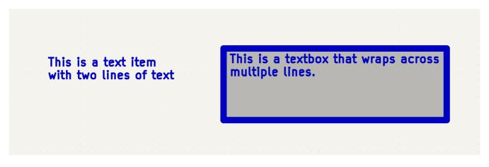
Both kinds of text item support multiline text and basic formatting features, but text boxes wrap text to fit in the outline and have additional formatting options. All text has adjustable fonts, color, size, bold and italic emphasis, left and right alignment, and vertical and horizontal orientation. Text boxes additionally support horizontal centering, vertical alignment options, and colored borders and fill. NOTE
