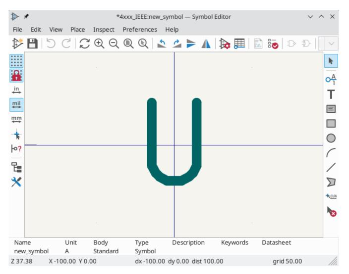
The blue cross in the center is the symbol anchor, which specifies the symbol origin i.e. the coordinates (0, 0). The anchor can be repositioned by selecting the 400 button and clicking on the new desired anchor position.
