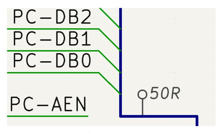
Net class directives are added with the  $\mathbf{Q}\mathbf{A}$  button in the right toolbar. They behave like labels, except that they cannot be used to name a net. The attached net is assigned a netclass according to the value of the directive's Net Class field. The Net Class field presents a dropdown list of all the net classes in the design.
