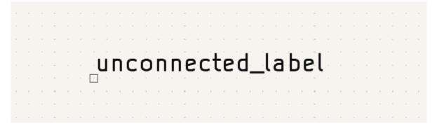
The connection point's position relative to the label text can be changed by choosing a different label orientation in the label's properties, or by mirroring/rotating the label.
